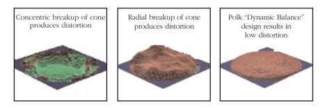
Laser Interferometry tests produced holographic "photos" of drivers in motion. The "bad" drivers are experiencing modal breakup that results in performance-robbing resonances. A "perfect" driver would look like a cake (flat on top), more, like the photo on the right.
